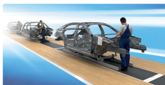
Das Skid Transfer System
